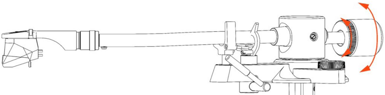
8. Rotate the loading dial on the counterweight to show zero **0** at the top center.
