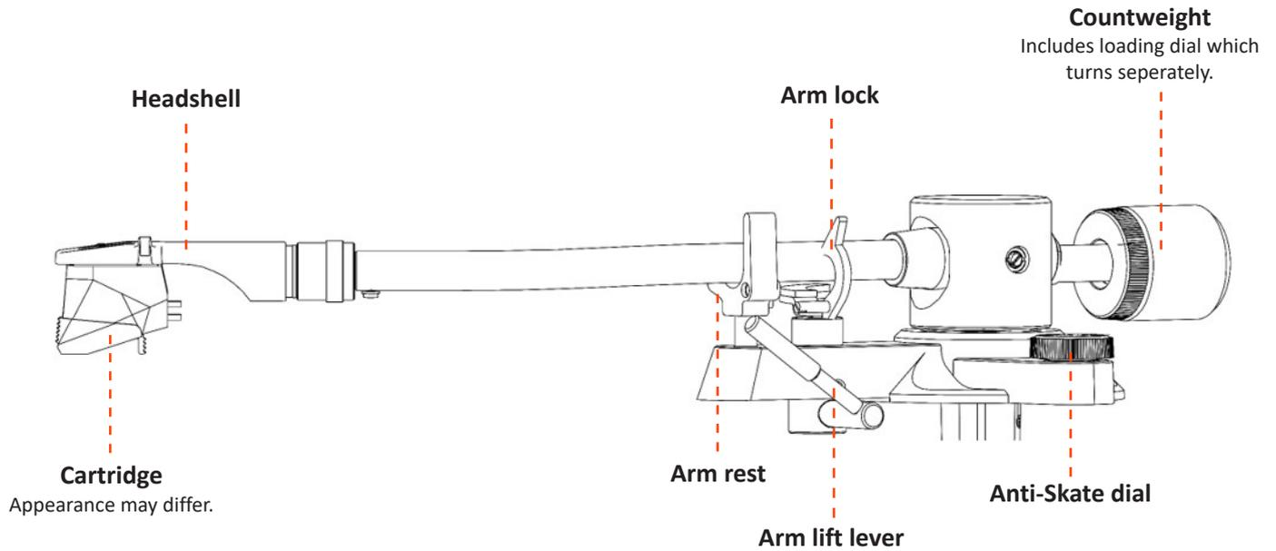
5. Rotate the counterweight slowly clockwise so it moves towards the back
