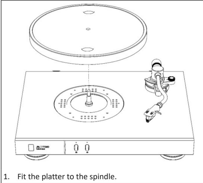
1. Fit the platter to the spindle.
