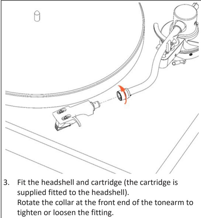
3. Fit the headshell and cartridge (the cartridge is supplied fitted to the headshell).
